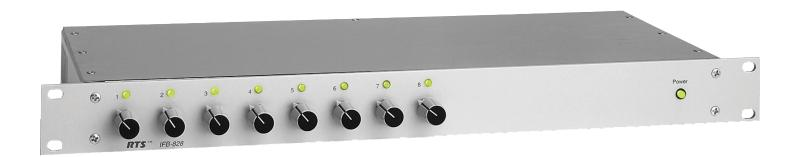
The IFB-828 interfaces up to eight (8) RTS Systems' Model IFB-325, 4020, or 4030 IFB beltpacks to any RTS Digital Matrix Intercom System, and it provides power to the beltpacks. The IFB-828 is used as a simple program interface to feed two (2) separate program sources to each of eight (8) 4020 or 4030 beltpacks (16 program sources to eight (8) beltpacks total).
